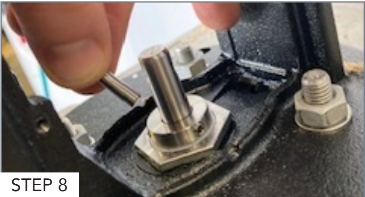
Slide the shaft pin out to gain access for deep well socket. (Do Not Lose Pin)
