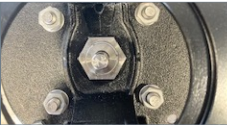
Top view for easy access of 36MM socket
