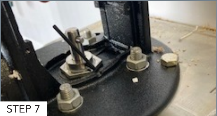
Loosen the set screws on the shaft collar, but do not fully remove the set screws. (2.5MM Allen Wrench)
